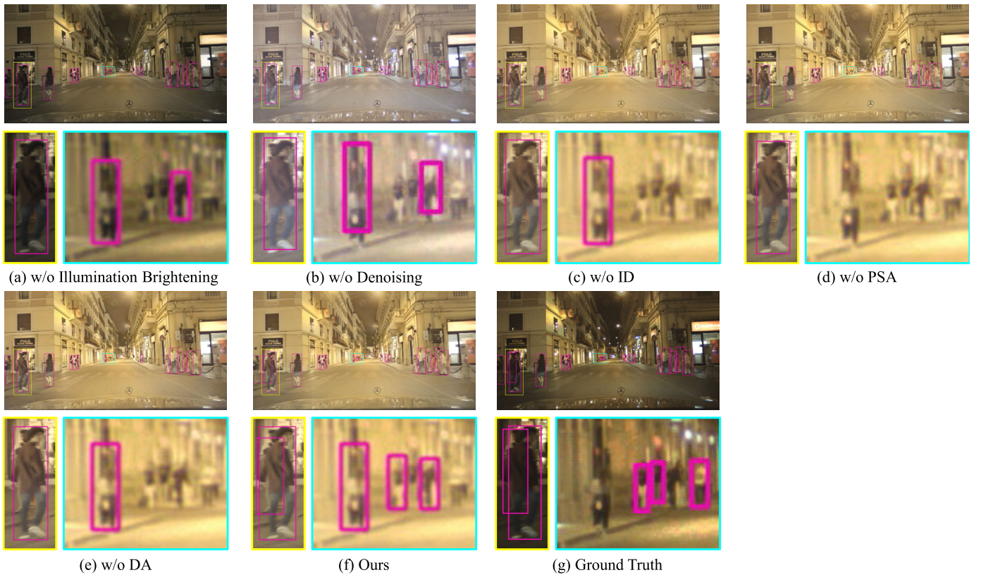
Fig. 6. Ablation study of individual components in the proposed method. (a) Illumination Brightening. (b) Illumination Difference-Aware Denoising Network. (c) Illumination Difference Guide. (d) Pseudo-Supervised Attention. (e) Degradation Alignment. (f) Ours. (g) Ground Truth. The pink bounding box represents the pedestrian class. Zoom in for better view.
